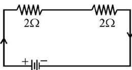
What will be the resultant resistance in the given electric circuit?
